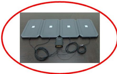
***Remark : The space between the antennas should be more than 20 cm, so that the tag's information can be shown on located antenna. Otherwise, tags would be read from other closed antenna. Space can be ignored if the application doesn't need tag's location information on located antenna.***
