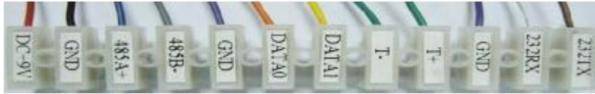
Figure 2 NFC-9601A reader wiring
